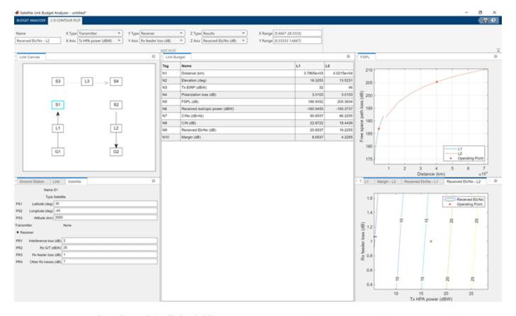
You can directly modify all the fields (Name, X Type, X Axis, Y Type, Y Axis, Z Type, Z Axis, X Range and Y Range) that appear in the 2-D Contour Plot tab. To access these fields for L1, in the lower-right pane, select the Received Eb/No - L1 tab.
