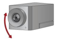
outPitch = campitch(viewer, \_\_\_\_) returns the pitch angle of the camera. If the second input is
