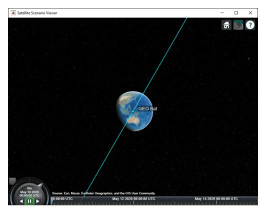
Add a ground track of the satellite to the visualization and adjust how much of the future and history of the ground track to display.
