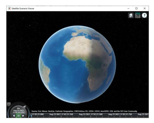
In the Satellite Scenario Viewer, set the latitude and longitude of the camera to -30 degrees and the height of the camera to 30,000 km.
