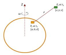
Consider that the positions of the source and the target are in International Terrestrial Reference Frame (ITRF).
