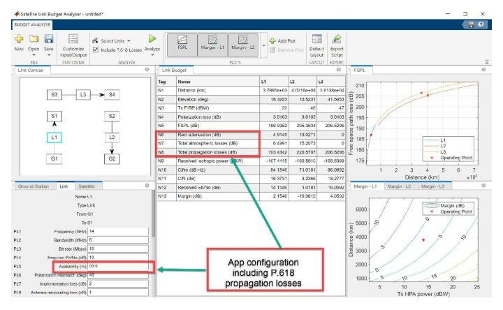
In this app, Total atmospheric losses (tag N7) calculation with P.618 propagation model assumes the antenna type as parabolic.
