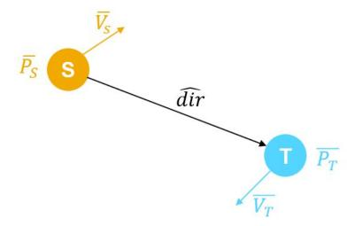
The unit vector from the source to the target is  $\widehat{dir} = \frac{\overline{P_T} - \overline{P_S}}{\|\overline{P_T} - \overline{P_S}\|}$ , where  $\|\|$  indicates the Euclidean norm.
